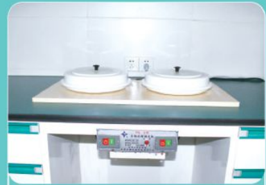
金相试样抛光机 Metallographic sample polishing machine
