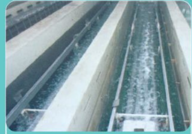
酸洗钝化处理 Pickling and passivation
