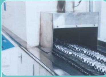
超声波清洗 Ultrasonic cleaning
