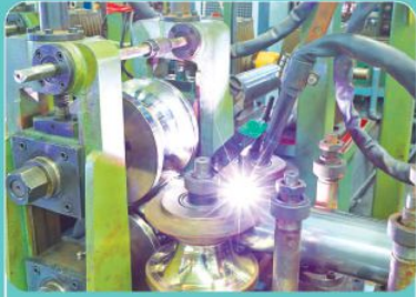
气体焊接保护 Gas welding protection
